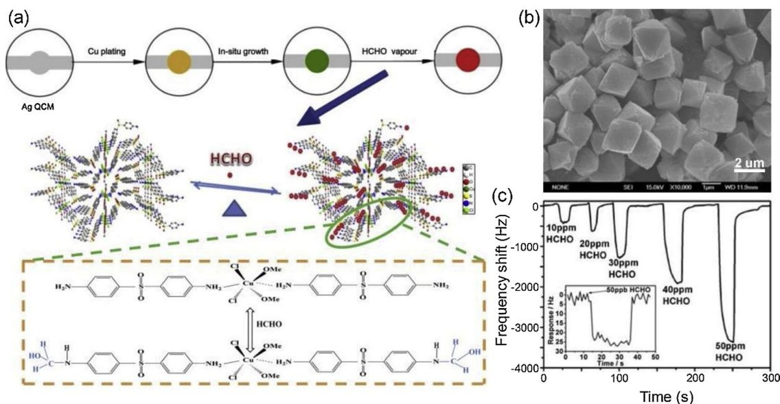
**Fig. 6.** (a) Scheme of the fabrication process of the complex based QCM gas sensor via situ growth method and specific capturing mechanism of HCHO molecules. (b) SEM image of the as-synthesized complex. (c) Typical sensor responses versus formaldehyde of various concentrations of 10, 20, 30, 40, 50 ppm, as well as 50 ppb at 298 K (Reused with permission from [56]. Copyright (2017) Elsevier).
