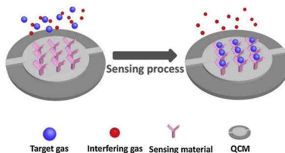
Fig. 3. The sensing process of the gas sensors based on QCM.
