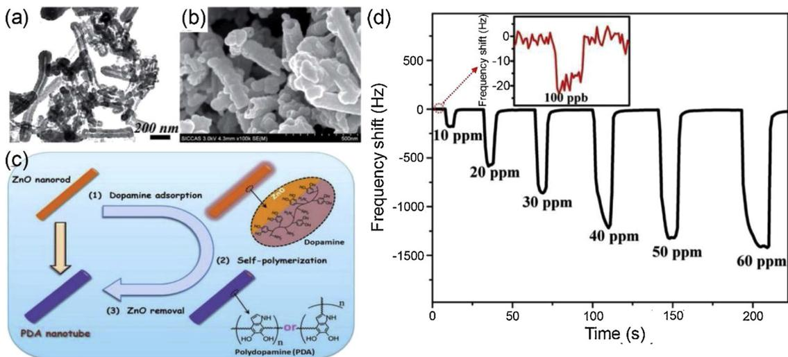
**Fig. 8.** (a) TEM image of the hollow PDA nanotubes. (b) SEM image of the hollow PDA nanotubes. (c) Roadmap of the synthesis procedure of hollow PDA nanotubes. (d) Real-time dynamic response curve of PDA based sensor exposure to HCHO with increasing concentration at room temperature. The inset shows the sensing response to 100 ppb HCHO (Reused with permission from [85]. Copyright (2016) Royal Society of Chemistry).
