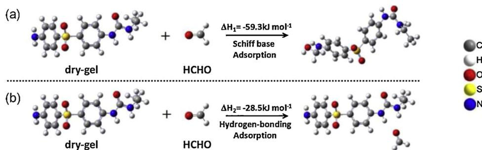
Fig. 15. The Gaussian simulations of Schiff base adsorption between HCHO molecule and dry-gel (Reused with permission from [57]. Copyright (2017) Elsevier).
