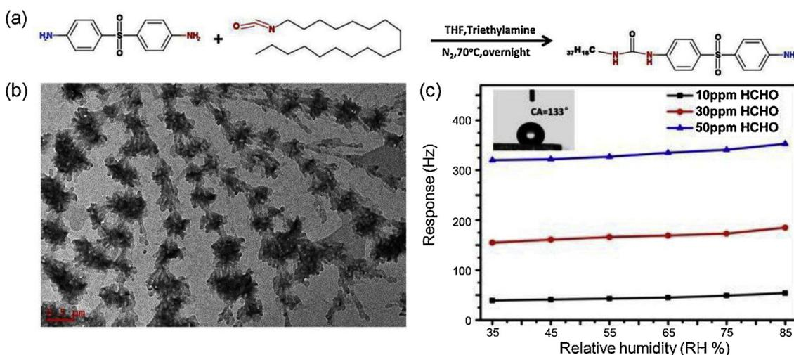
**Fig. 7.** (a) The synthesis process of the urea material. (b) TEM image of the dry-gel. (c) The frequency response of dry-gel based QCM sensor exposed to 10, 30, and 50 ppm of formaldehyde at some common relative humidity environments. The inset shows the contact angle image of dry-gel based QCM (Reused with permission from [57]. Copyright (2017) Elsevier).
