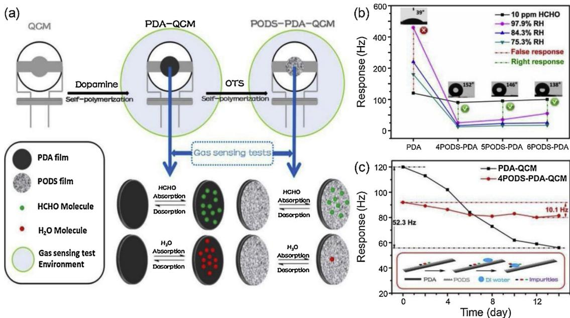
**Fig. 9.** (a) Scheme of the experiment we design. (b) False response region of PDA-QCM and right response region of PODS covering PDA-QCMs. (c) Sensing results are obtained with an interval of two weeks for evaluating long term stability of 4PODS-PDA-QCM towards 10 ppm HCHO. The inset shows the reason for long-term stability (Reused with permission from [35]. Copyright (2018) Elsevier).
