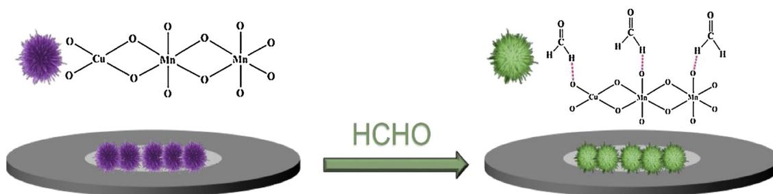
Fig. 10. Schematic illustration of the HCHO sensing mechanism of the as-prepared copper-manganese composite oxide.
