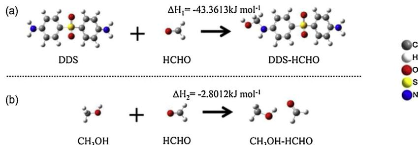
Fig. 14. Optimized geometries and interactions between HCHO molecule and ligands (a) DDS and (b)  $\text{CH}_3\text{OH}$  (Reused with permission from [56]. Copyright (2017) Elsevier).
